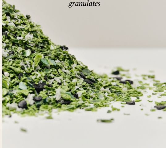
Plastic beer kegs Empty beer kegs are cleaned and processed into ready-to-use plastic granulates
