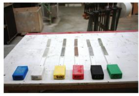
For grinding the edges, use a sand paper block with a graining of 60 to 500.
