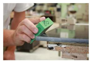
2. The sand paper block is to be used for final forming and polishing of the bevel and front edge, as shown in the picture.
