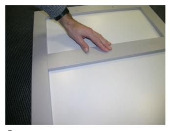
3 Glue bar in position and press down firmly.
